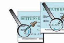
In order to get these results we use a thin laser beam which perforates the paper with small but visible points, which reproduce, in their arrangement, the numbers or letters that make up the data that have to be protected
